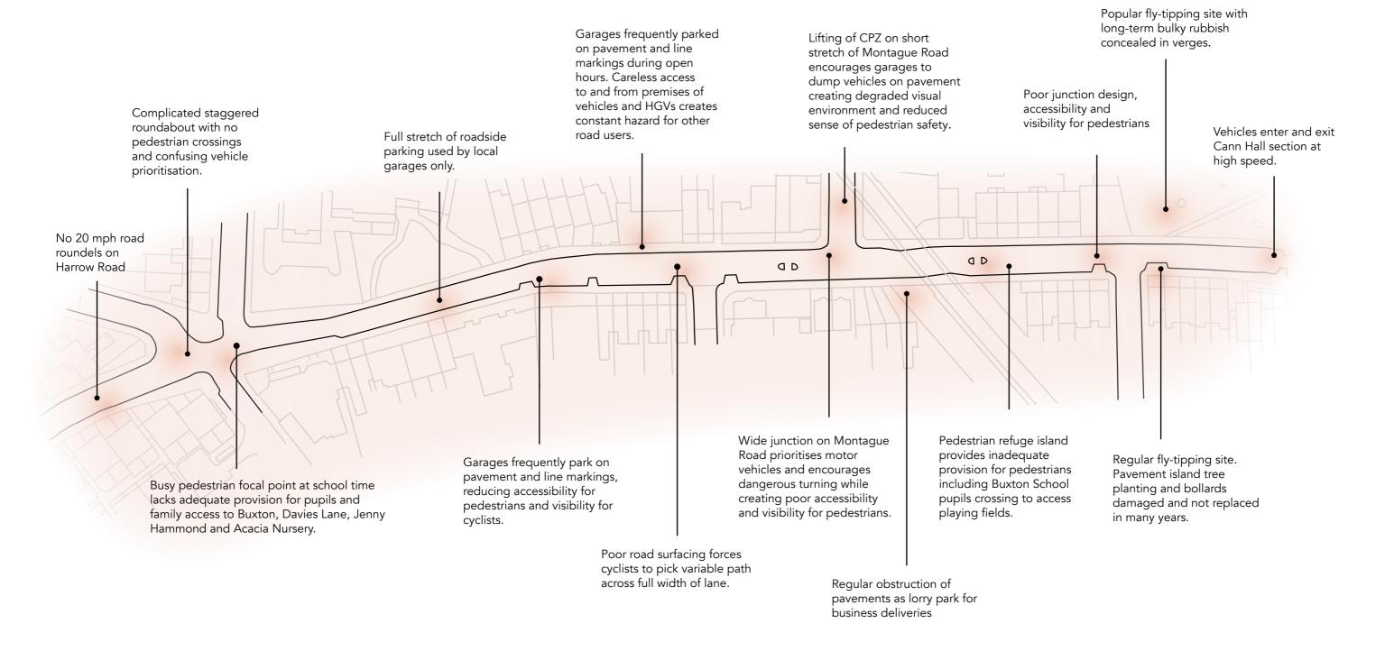
Characterised by a long straight carriageway, with no speed signage throughout section and very poor surfacing. Poor visual sense of public space dominated by local garages blocking footpaths and carriageways, impeding and endangering safe access for all users. Irregular road widths, parking and traffic calming create hazardous pinch-points along entire stretch.
