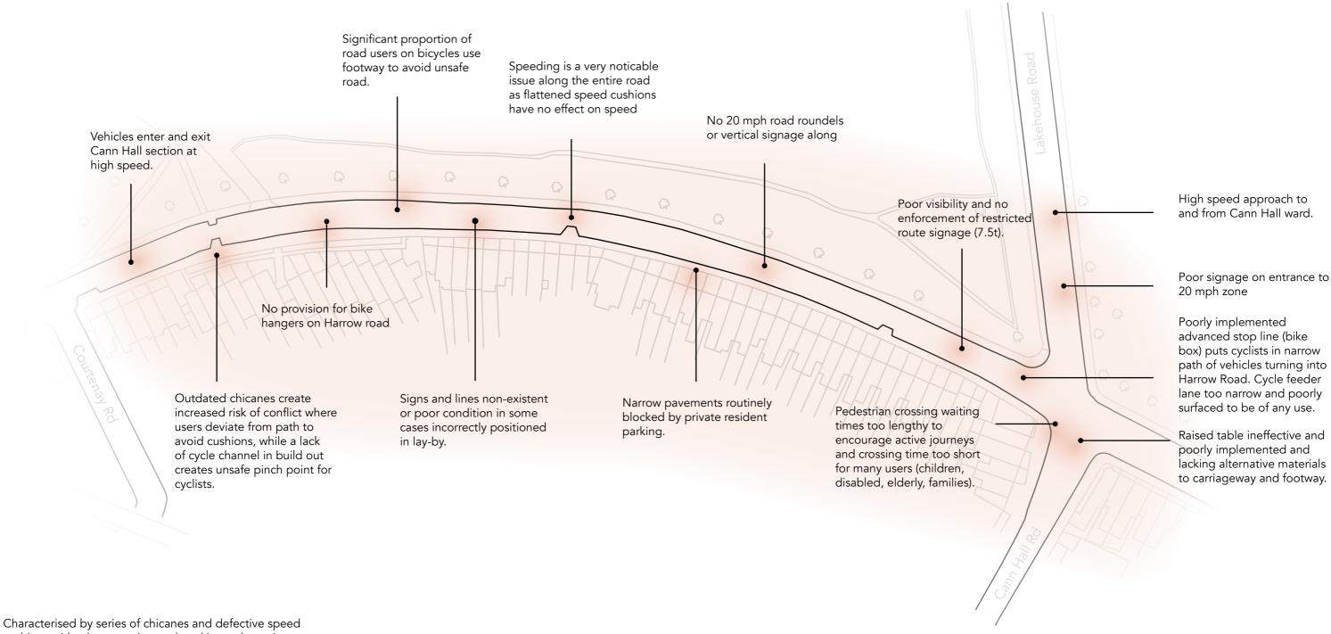
Characterised by series of chicanes and defective speed cushions with a long continuous bend in road creating poor visibility especially for east west journeys. No speed signage throughout section. Attractive roadside verge and sightlines across Wanstead flats poorly utilised with limited engagement or provision for active accessibility.
